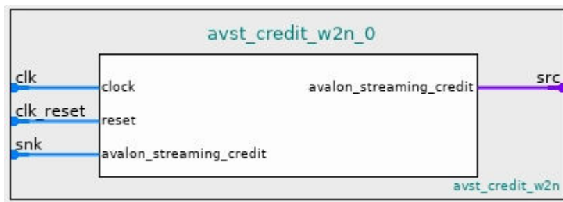
Figure 216. Avalon Streaming Credit Wide to Narrow Adapter
