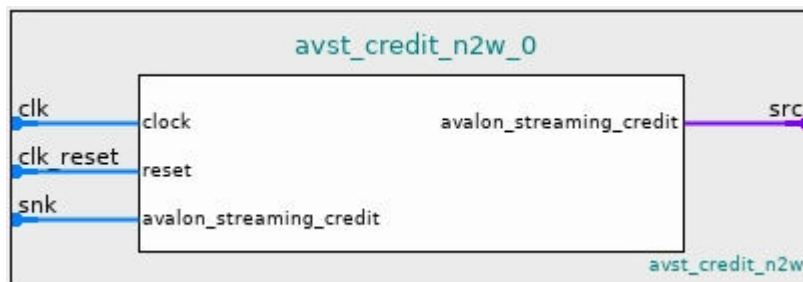
Figure 218. Avalon Streaming Credit Narrow to Wide Adapter
