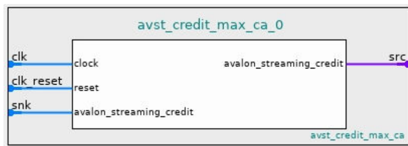
Figure 220. Avalon Streaming Credit Max Credit Adapter
