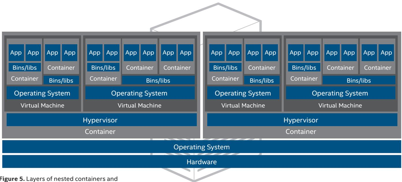
**Figure 5.** Layers of nested containers and hypervisor-based virtual machines.
