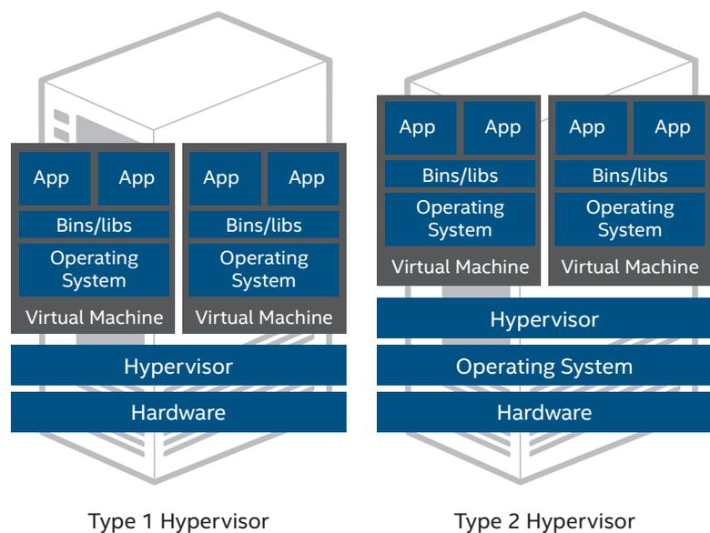
Figure 2. Virtualization based on Type 1 and Type 2 hypervisors.
